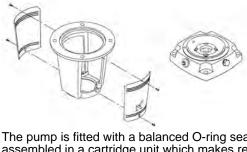
The pump is fitted with a balanced O-ring seal unit with a rigid torque-transmission system. This seal type is assembled in a cartridge unit which makes replacement safe and easy. Due to the balancing, this seal type is suitable for high-pressure applications. The cartridge construction also protects the pump shaft from possible wear from a dynamic O-ring between pump shaft and shaft seal.
