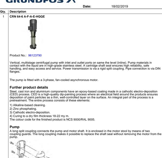
The motor stool connects the pump head and motor. The pump head has a combined 1/2" priming plug and vent screw.
