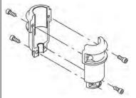
The motor stool connects the pump head and motor. The pump head has a combined 1/2" priming plug and vent screw.
