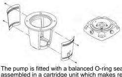
The pump is fitted with a balanced O-ring seal unit with a rigid torque-transmission system. This seal type is assembled in a cartridge unit which makes replacement safe and easy. Due to the balancing, this seal type is suitable for high-pressure applications. The cartridge construction also protects the pump shaft from possible wear from a dynamic O-ring between pump shaft and shaft seal.
